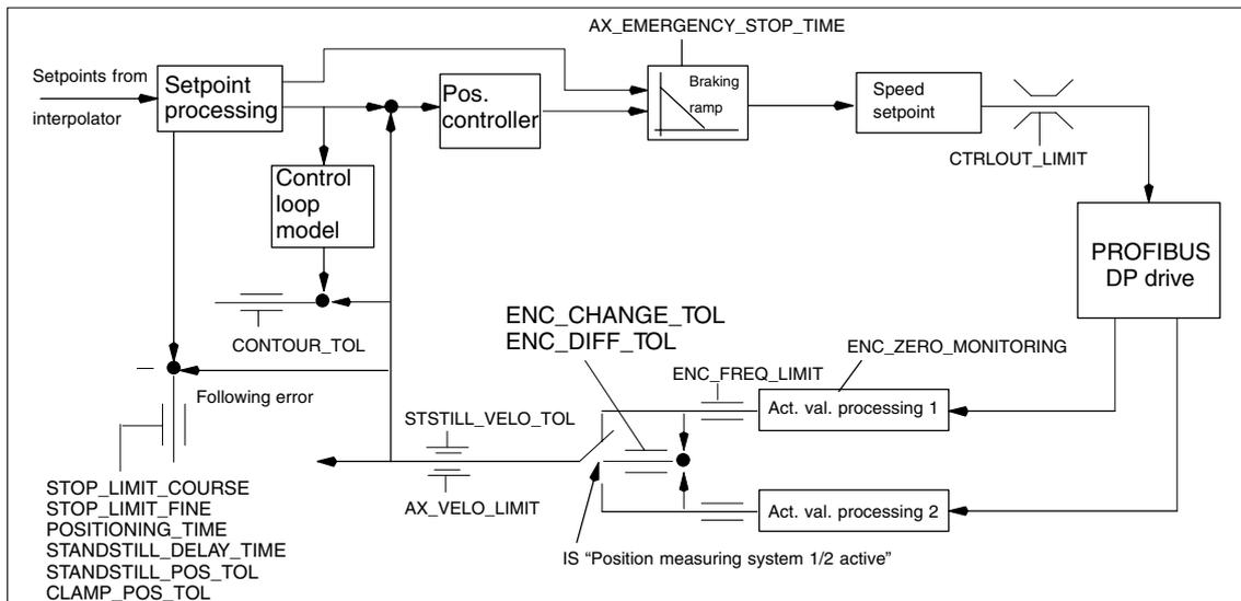
Fig. 11-22 Monitoring for SINUMERIK 840Di sl
