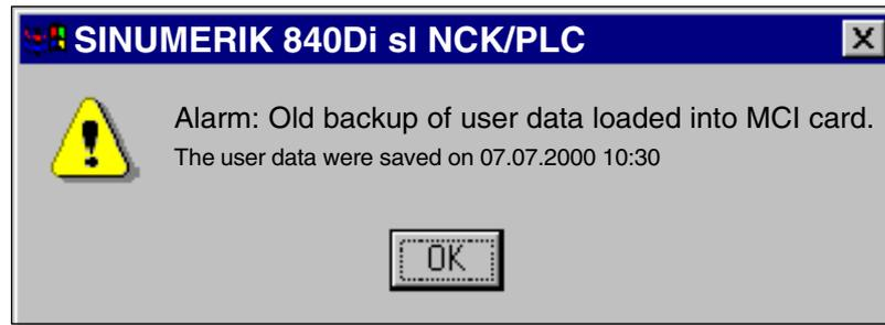
In addition, an NC alarm is output, which is displayed on the appropriate user interface of the SINUMERIK 840Di sl (840Di startup, HMI Advanced, etc.):
