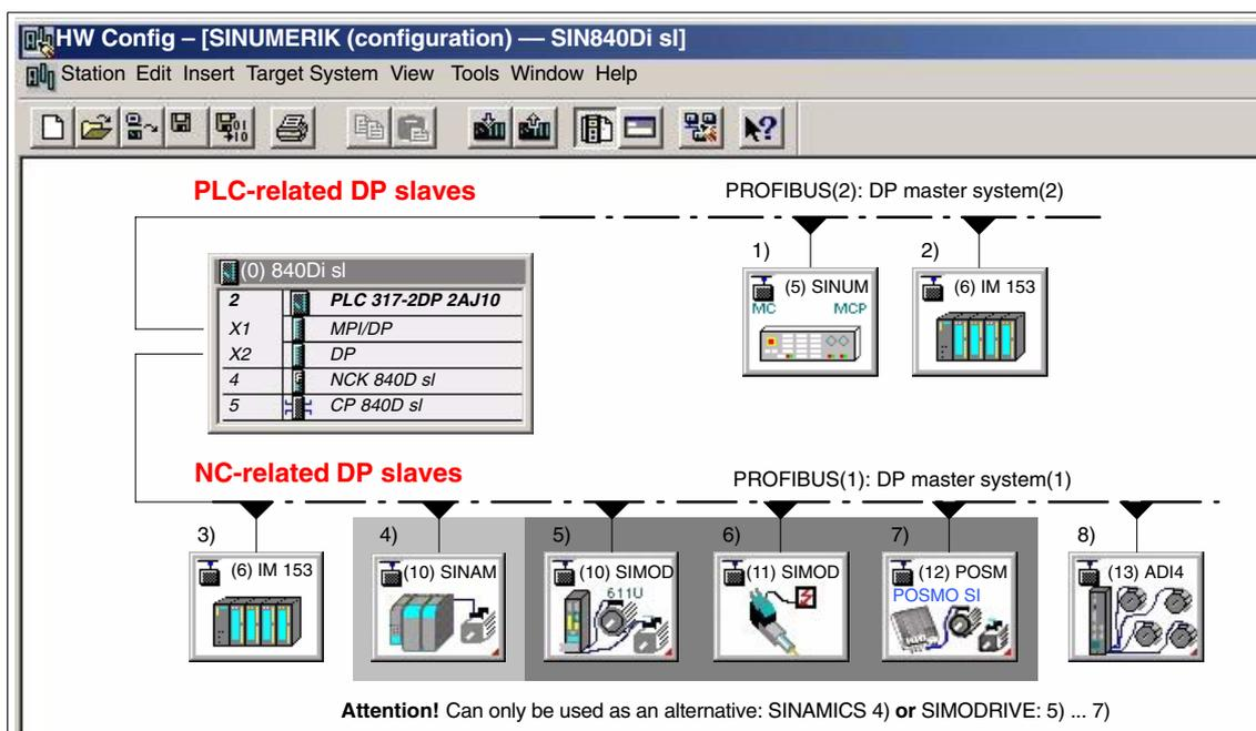
Fig. 8-6 Recommended distribution of DP slaves (schematic)
