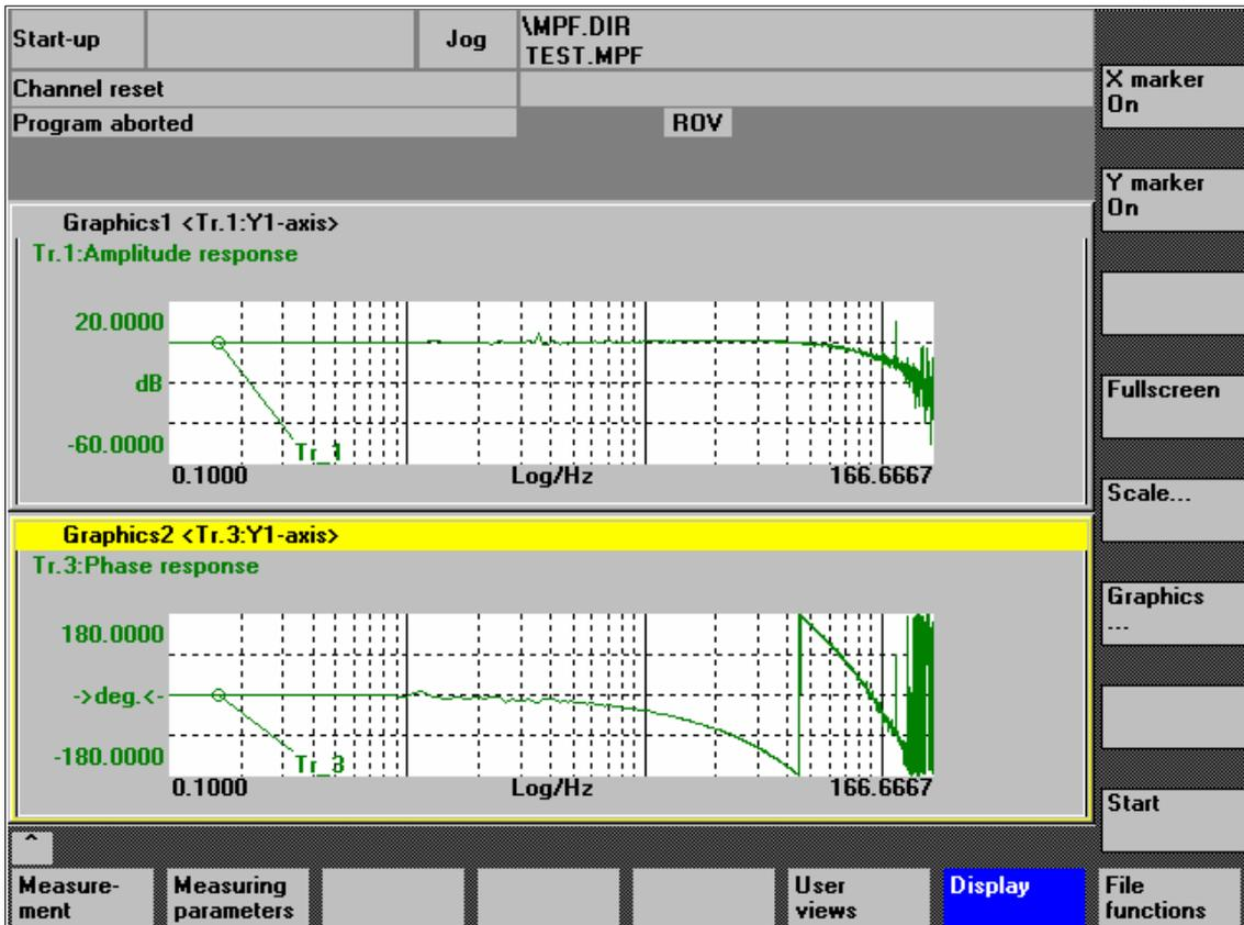
Fig. 14-2 Example: Measurement results of a reference frequency response measurement
