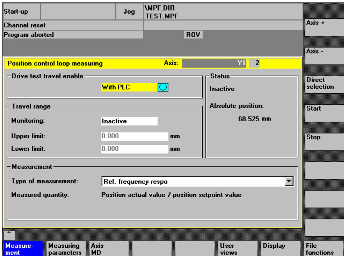
Fig. 14-1 Main menu: Position control loop measurement
