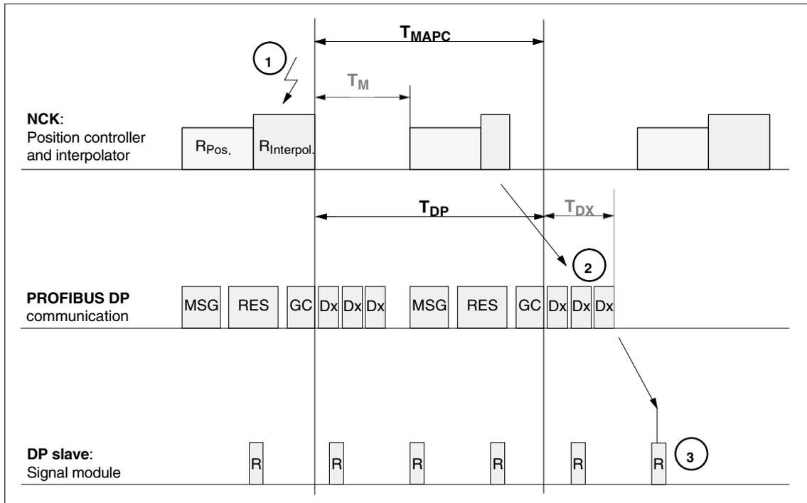
Fig. 11-32 Time response when outputting an output signal with optimized DP cycle
