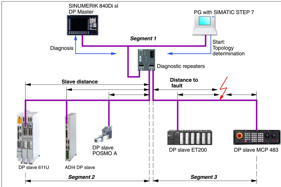
Fig. 8-24 Example: PROFIBUS topology with diagnostic repeater
