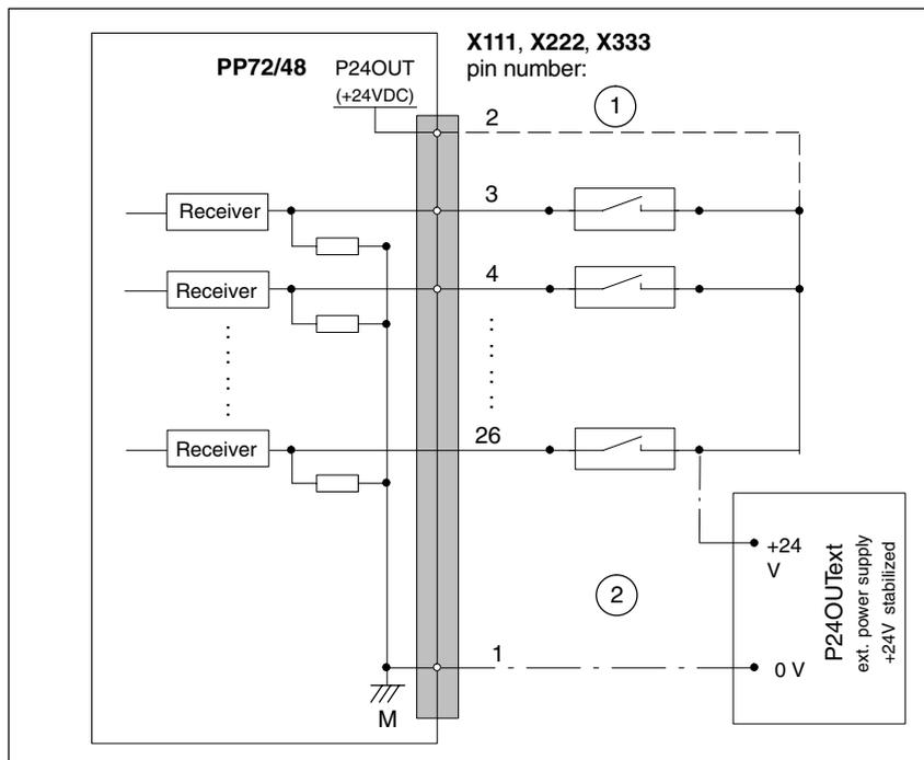
Fig. 2-21 Terminal assignment for the digital inputs
