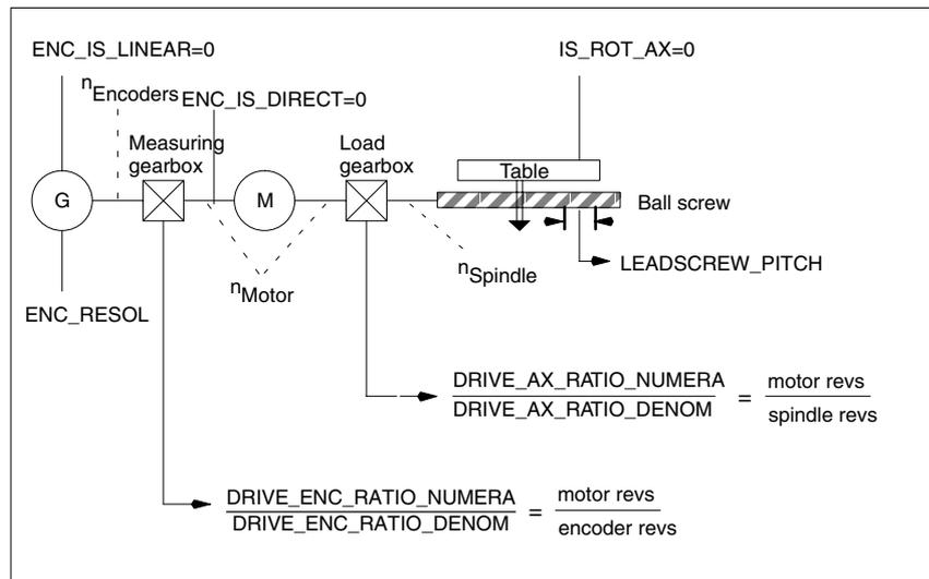
Fig. 11-5 Linear axis with encoder on motor
