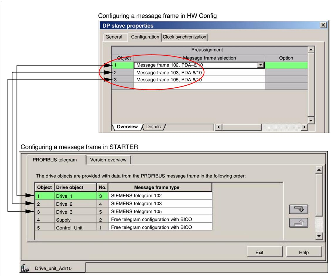
Fig. 8-21 Process data structure: HW Config and STARTER
