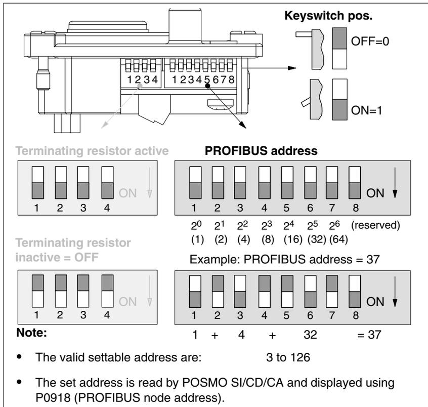
Fig. 10-2 Setting the PROFIBUS address and terminating resistor
