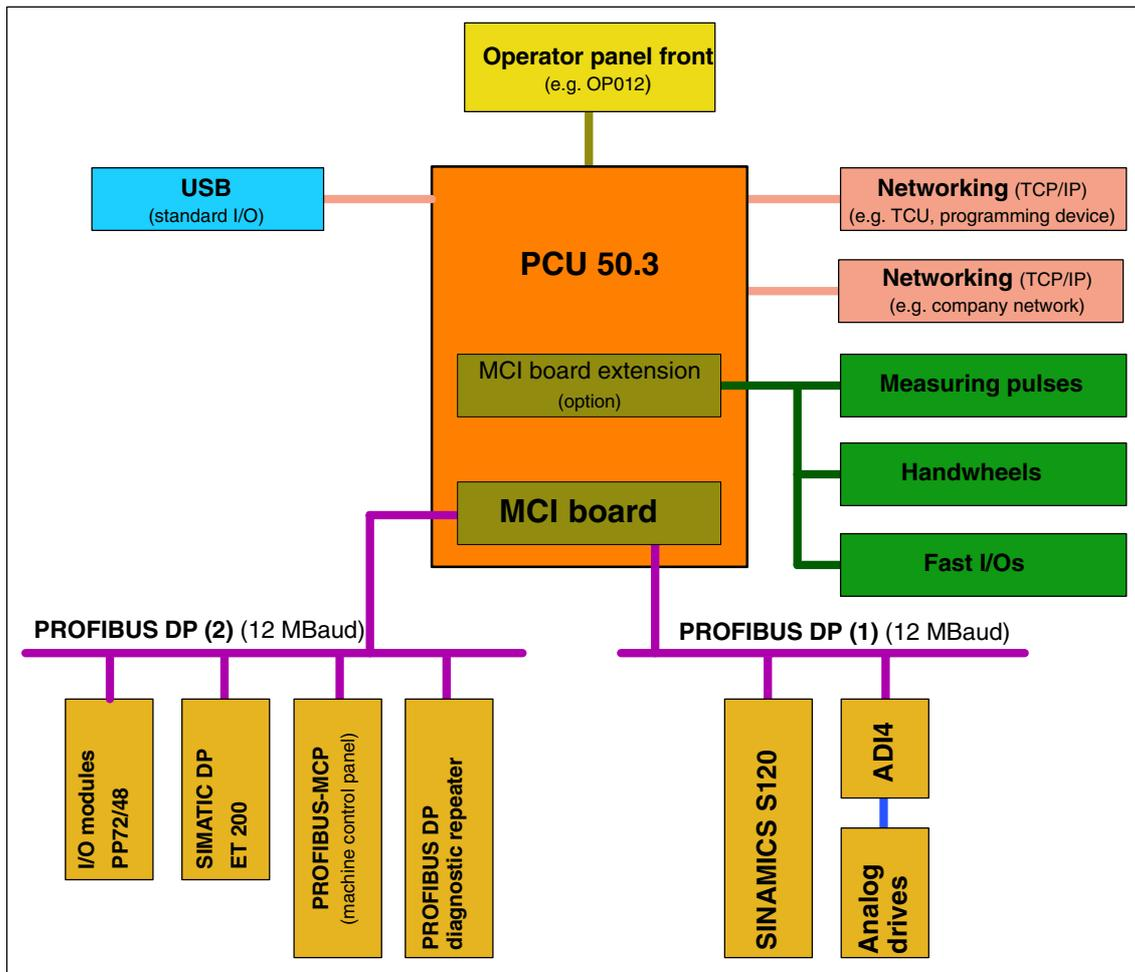
Fig. 1-1 System overview of SINUMERIK 840Di sl
