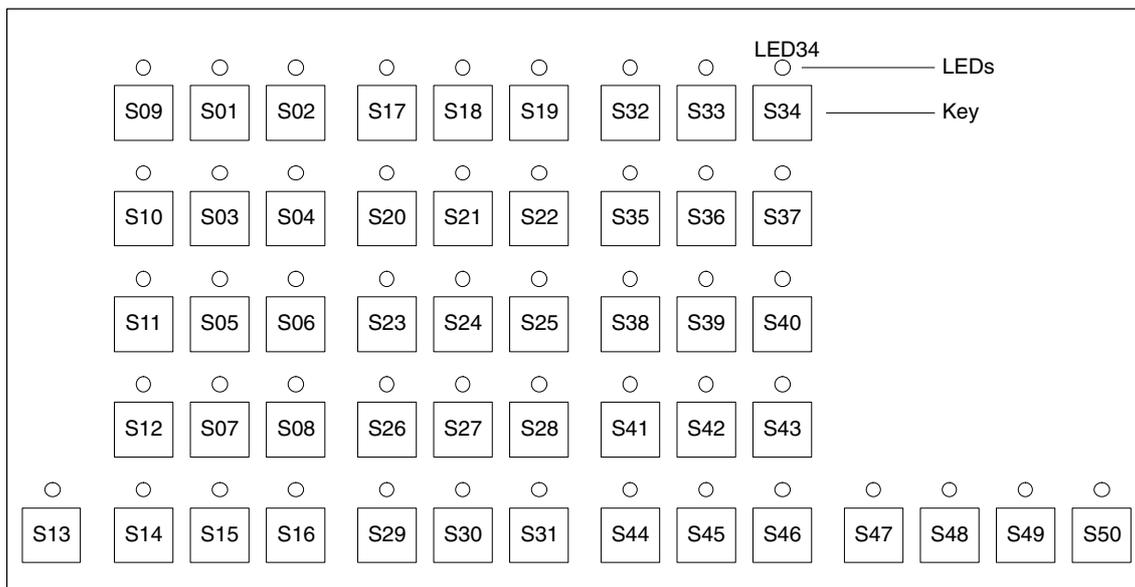
Fig. 8-20 MCP 483 keyboard layout (front view)
