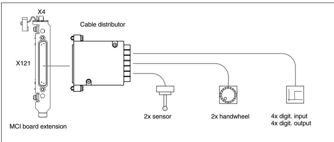
Fig. 3-7 SINUMERIK 840Di sl MCI board extension
