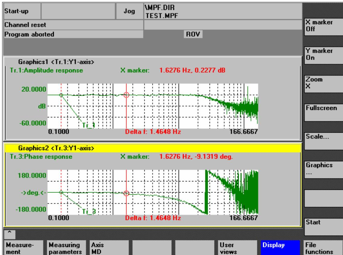
Fig. 14-6 Menu: Display of measurement with marker X = ON
