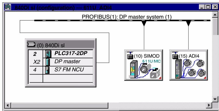
Fig. 11-12 Configuration: Axis with 2nd measuring system on ADI4
