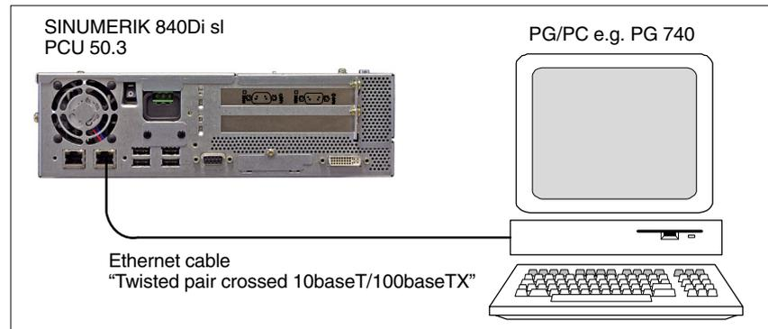
Fig. 16-1 PTP link: PCU 50.3 – External computer (PG/PC)
