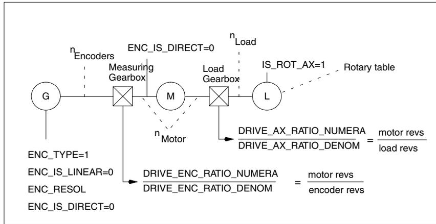
Fig. 11-7 Rotary axis with encoder on motor
