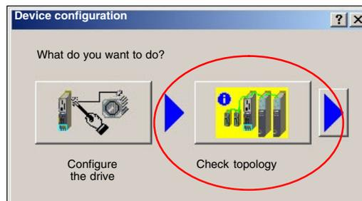
2. Compare the DRIVE-CliQ topology displayed in the STARTER with the topology of the drive unit.
