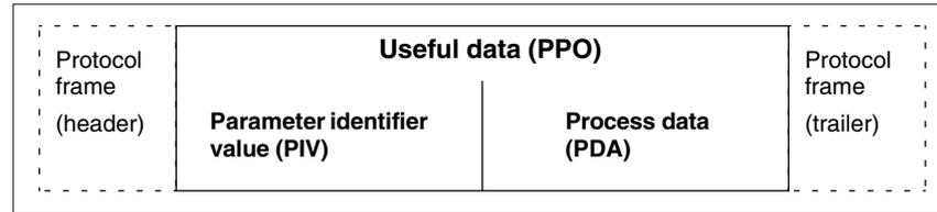
Fig. 8-1 Main message format for cyclic data transmission
