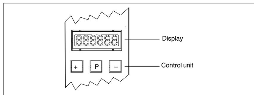
Fig. 10-1 Display and control unit
