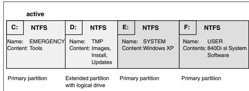
Fig. 16-3 Partitioning of the harddisk
