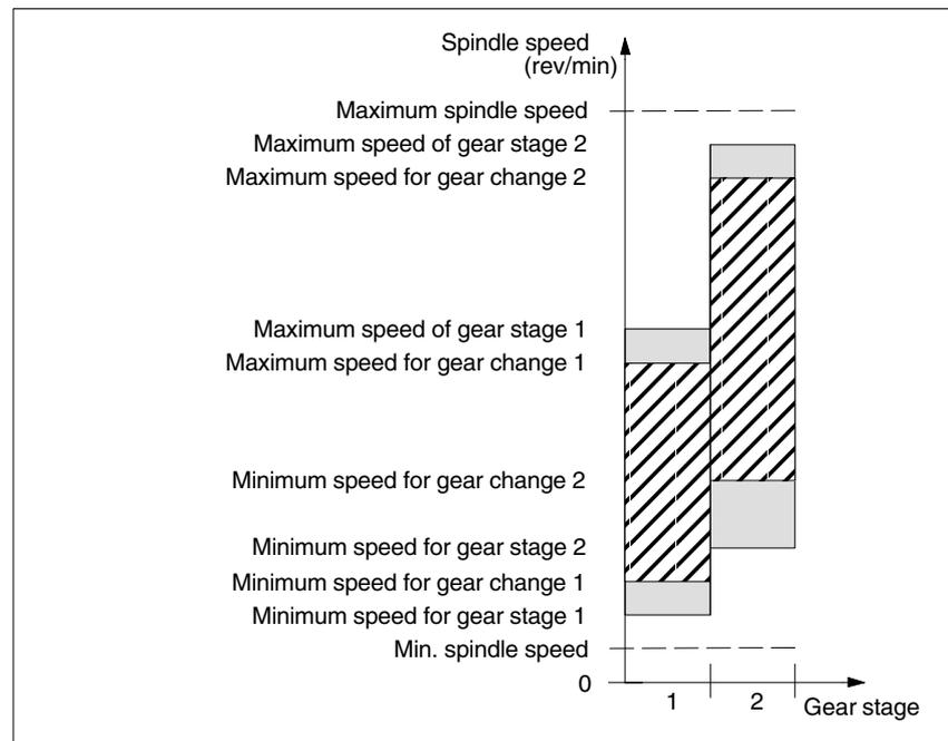
Fig. 11-27 Example for speed ranges for automatic gear stage selection (M40)
