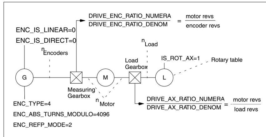
Fig. 11-11 Rotary axis with absolute value encoder on motor
