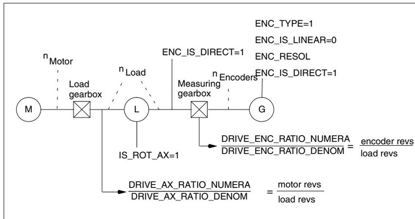
Fig. 11-8 Linear axis with encoder on the machine
