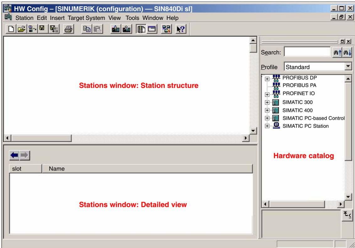
Fig. 6-4 HW Config: Names of the main areas
