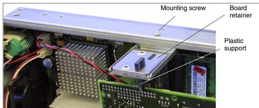
Fig. 2-4 Mounting of the module
