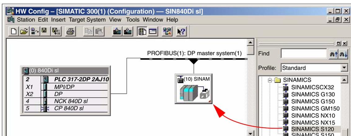
Fig. 8-5 HW Config: Inserting modules, e.g., SINAMICS S120
