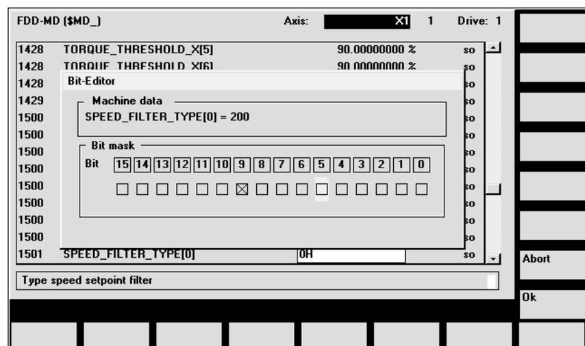
Fig. 11-1 Input screen form of the bit editor for HEX machine data
