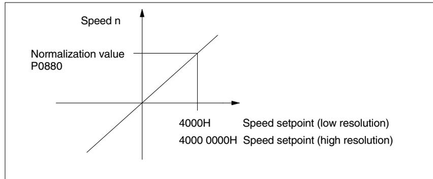
Fig. 11-28 Speed setpoint normalization
