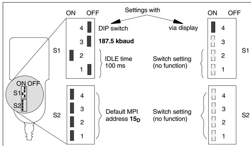
Fig. 7-14 Settings required on the HHU for SINUMERIK 840Di sl
