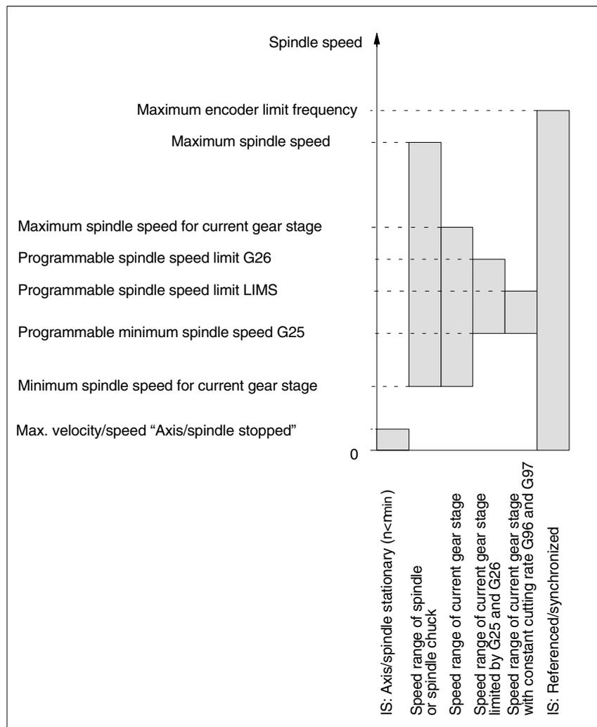
Fig. 11-30 Ranges of spindle monitoring functions/speeds
