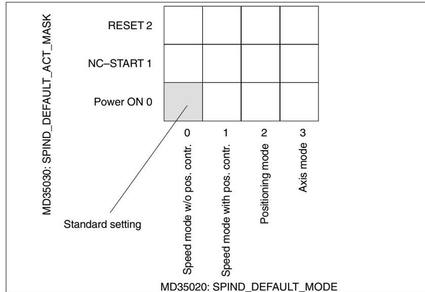
Fig. 11-26 Default setting of spindle mode
