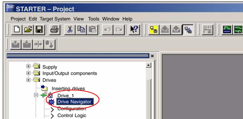
Then click in the drive navigator dialog on the button: "Device configuration" and in the device configuration dialog on the button: "Configure the drive".
