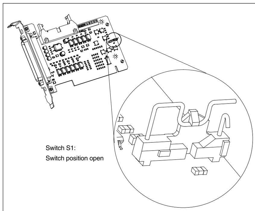
Fig. 2-7 Switch S1 switch position open (TTL handwheels)
