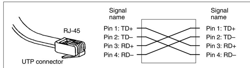
Fig. 16-2 Crossed Ethernet cable (twisted pair crossed 10baseT/100baseTX)
