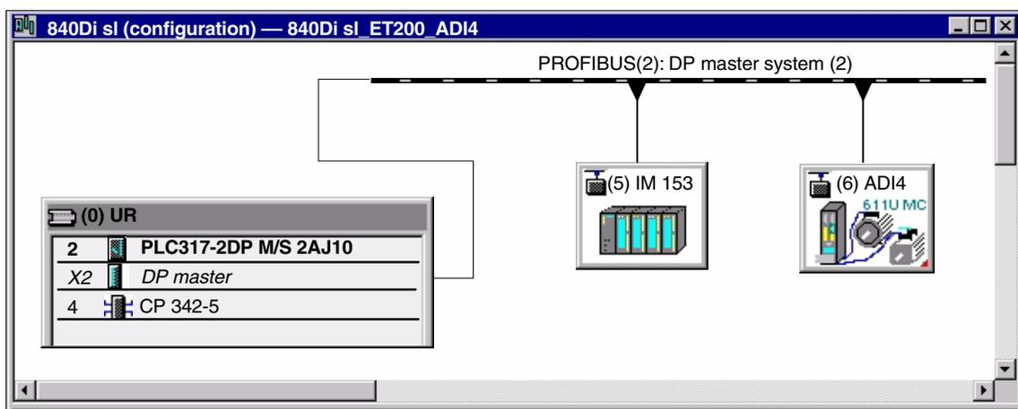
Fig. 11-33 Example configuration: SINUMERIK 840Di sl with ET200 and ADI4
