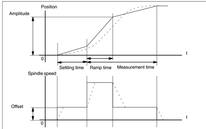
Fig. 14-5 Signal chart for position setpoint/ramp measuring function
