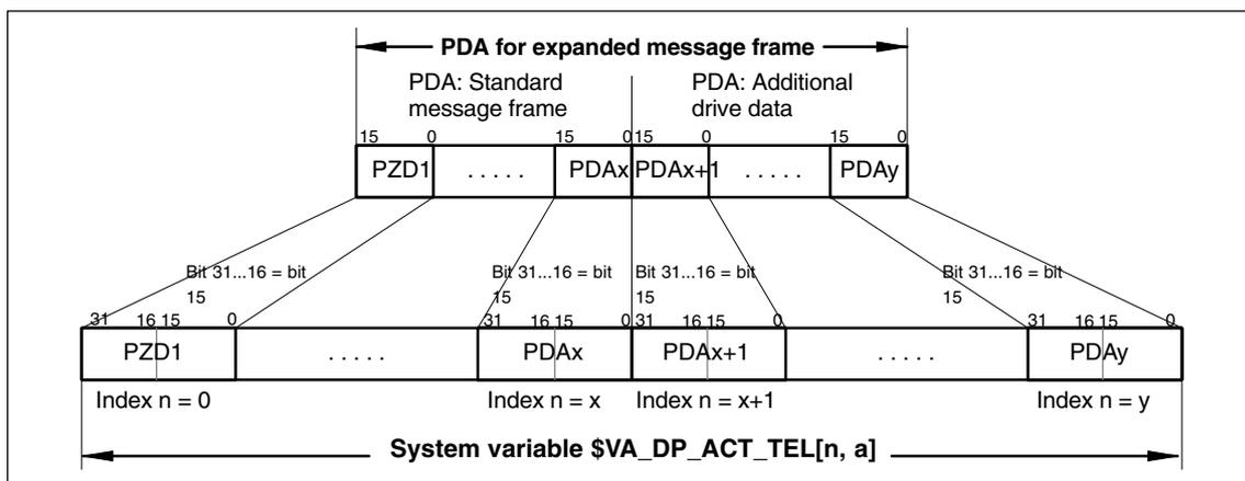
Fig. 18-2 Mapping principle: PDA on system variable \$VA\_DP\_ACT\_TEL
