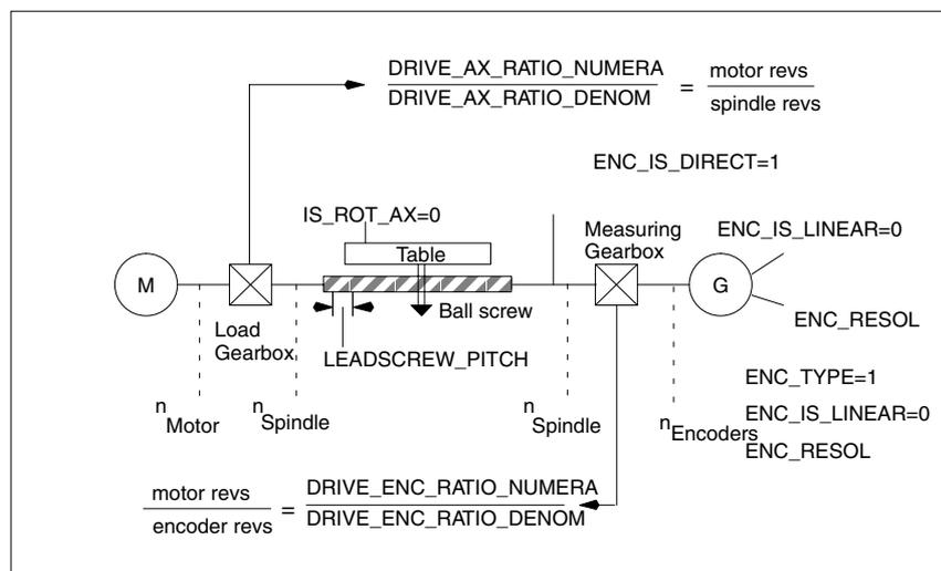
Fig. 11-6 Linear axis with encoder on the machine
