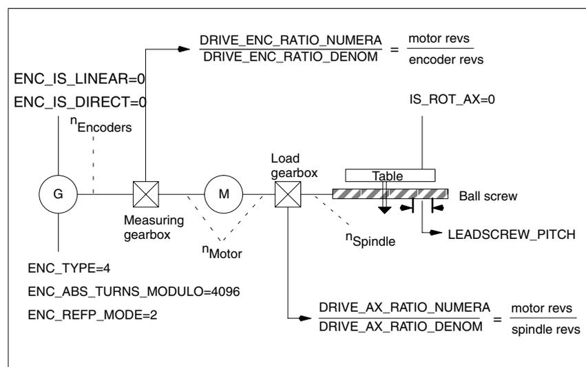
Fig. 11-10 Linear axis with absolute value encoder on motor
