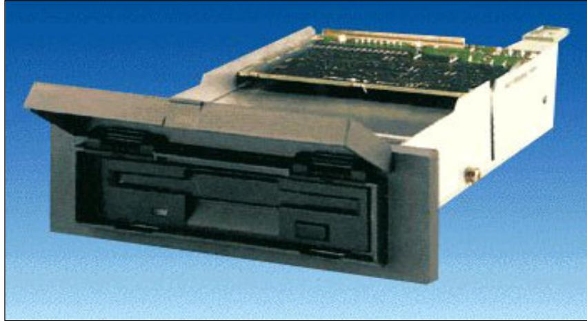
Fig. 2-16 External 3.5" floppy disk drive and 3.5" with USB interface
