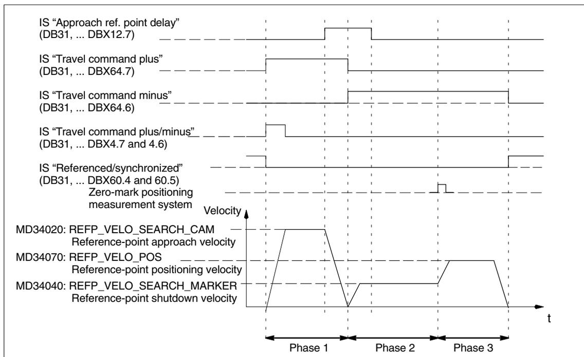
Fig. 11-23 Signal chart: Referencing with an incremental measuring system (principle)
