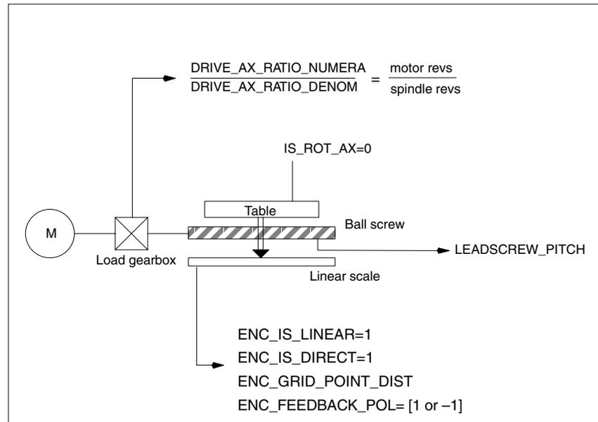
Fig. 11-9 Linear axis with linear scale
