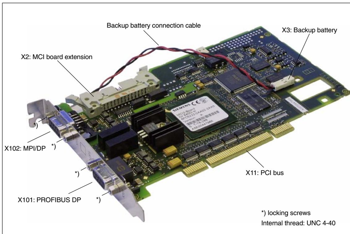
Fig. 2-1 Module: MCI2 board for 840Di sl
