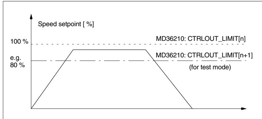
Fig. 11-20 Speed setpoint monitoring
