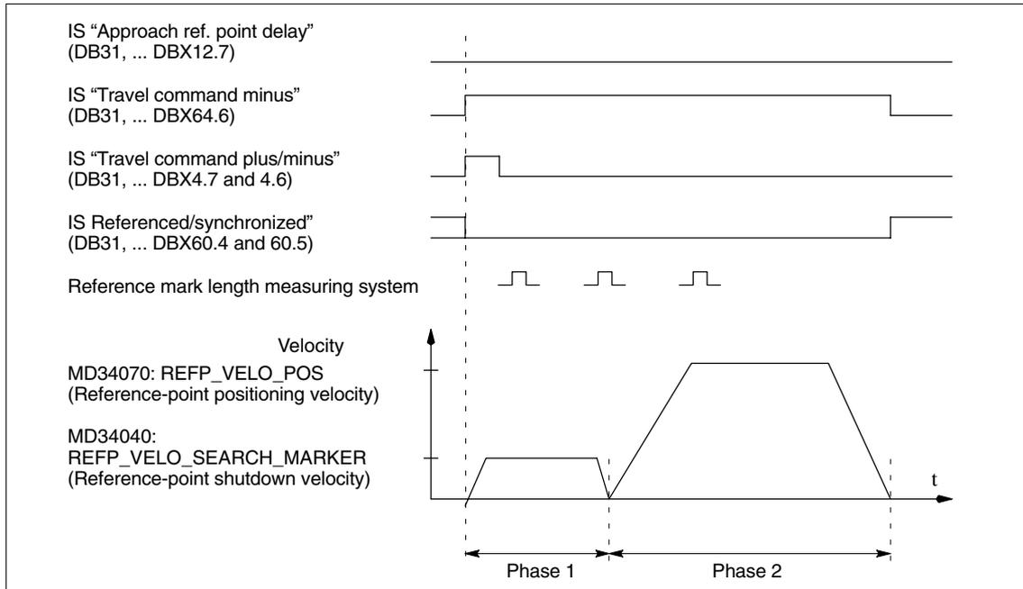
Fig. 11-24 Signal chart: Distance-coded reference marks (principle)
