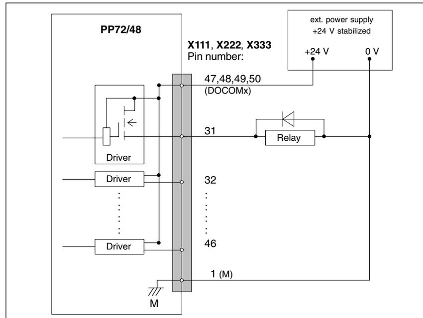
Fig. 2-22 Terminal assignment for the digital outputs
