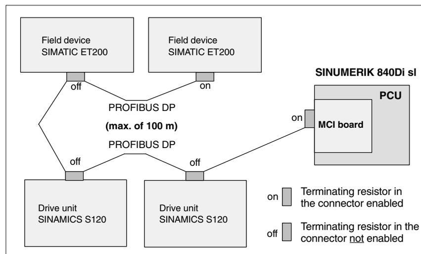
Fig. 8-3 Example of a PROFIBUS DP network installation
