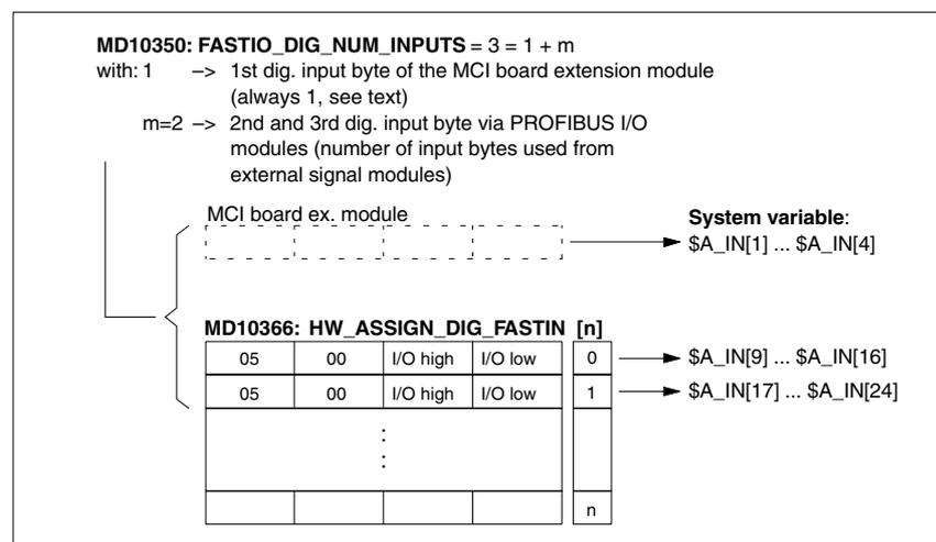
Fig. 11-31 Configuration example: 3 digital input bytes
