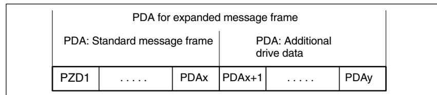
Fig. 18-1 Standard message frame with additional process data (PDA)
