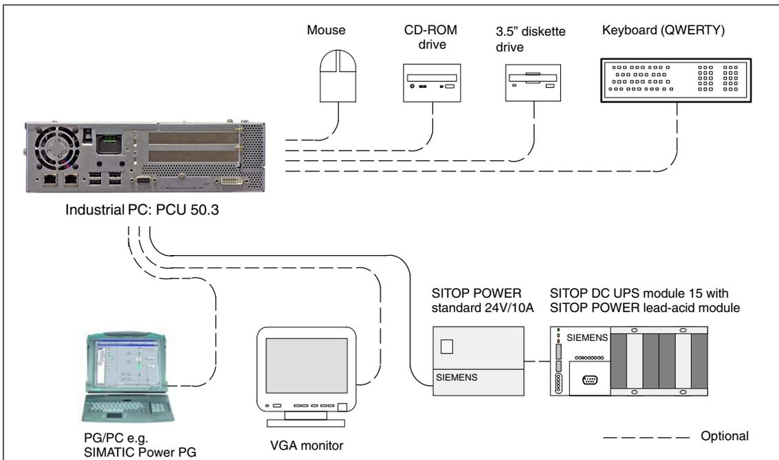
Fig. 3-4 System overview of SINUMERIK 840Di sl PCU components (as a diagram)
