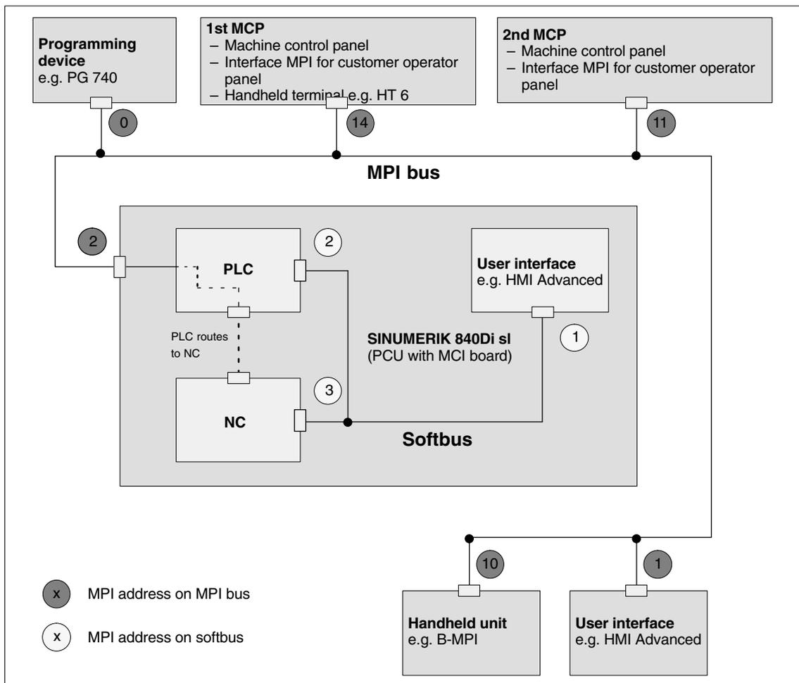
Fig. 7-5 Recommended MPI addresses for SINUMERIK 840Di sl
