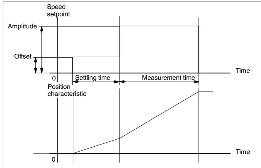
Fig. 14-3 Setpoint signal for speed control loop/step response measuring function
