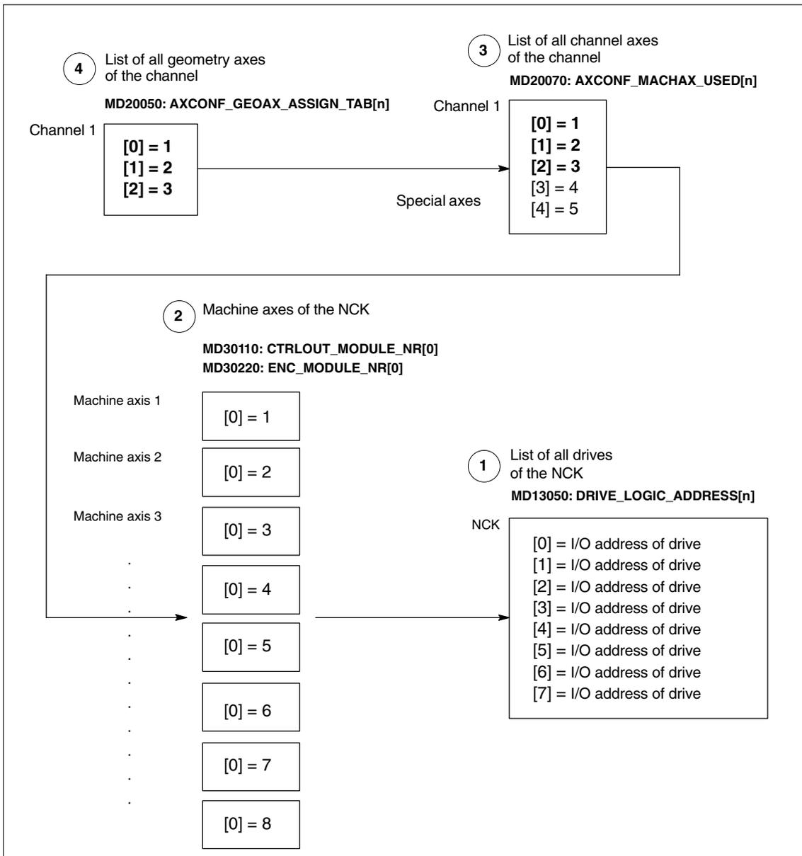
Fig. 11-4 Axis assignment
