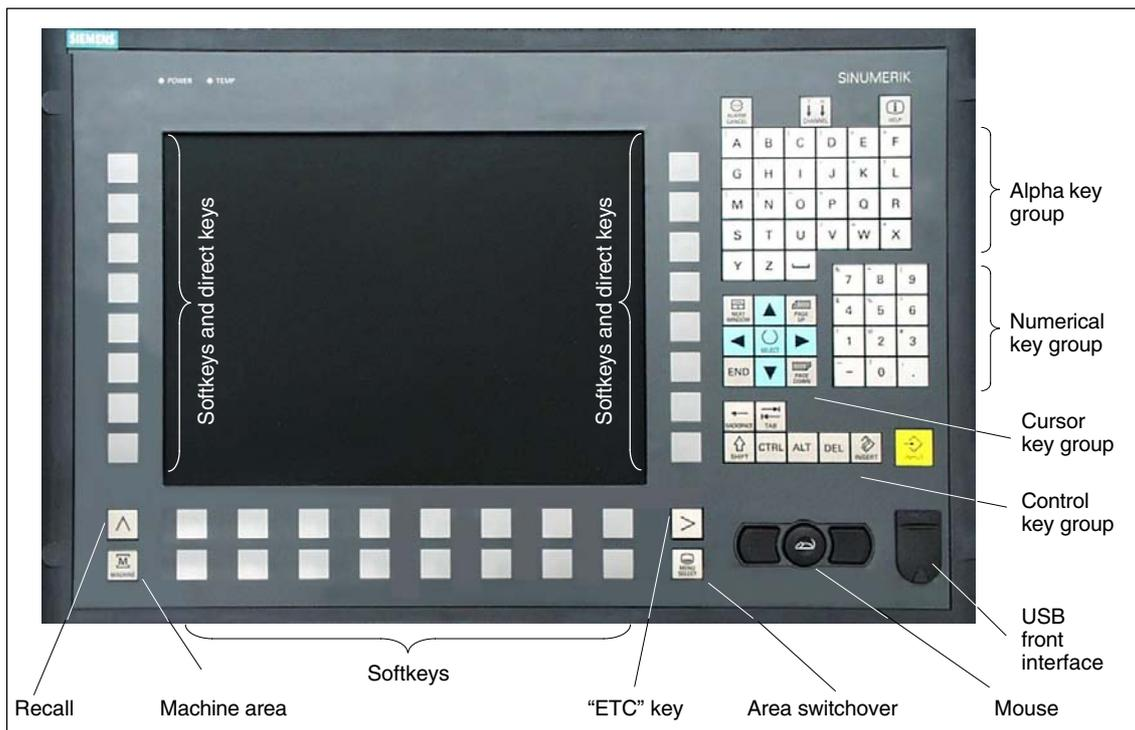
Fig. 2-14 View of OP 012 operator panel front
