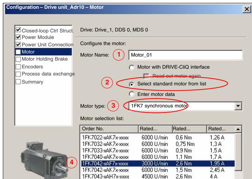
Select the motor type, e.g., 1FK7 synchronous motor (3), from the drop-down list and the current motor from the corresponding list based on the order number (MLFB) (4).
