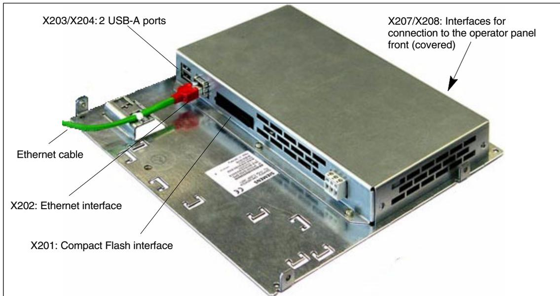
Fig. 2-15 TCU with Ethernet cable plugged in
