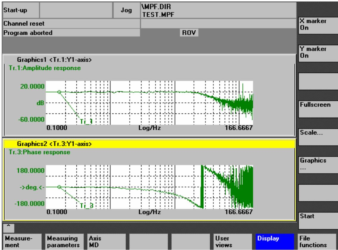
Fig. 14-4 Example: Measurement results of a reference frequency response measurement
