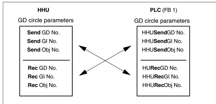
Fig. 7-18 Crosswise coincidence of GD circle parameters
