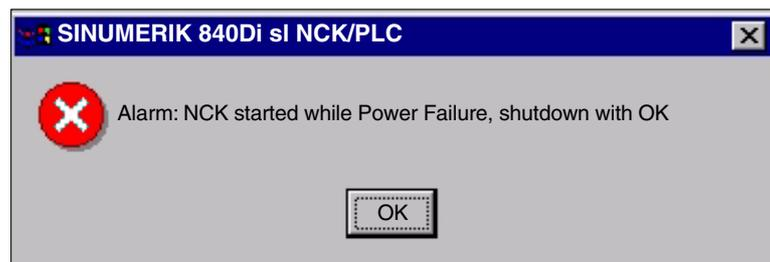
This system response ensures that an error in the protection circuit of the MCI board extension module or in the configuration of the shutdown signal does not result in an endless loop (power-up > shutdown signal > power-up > etc.).
