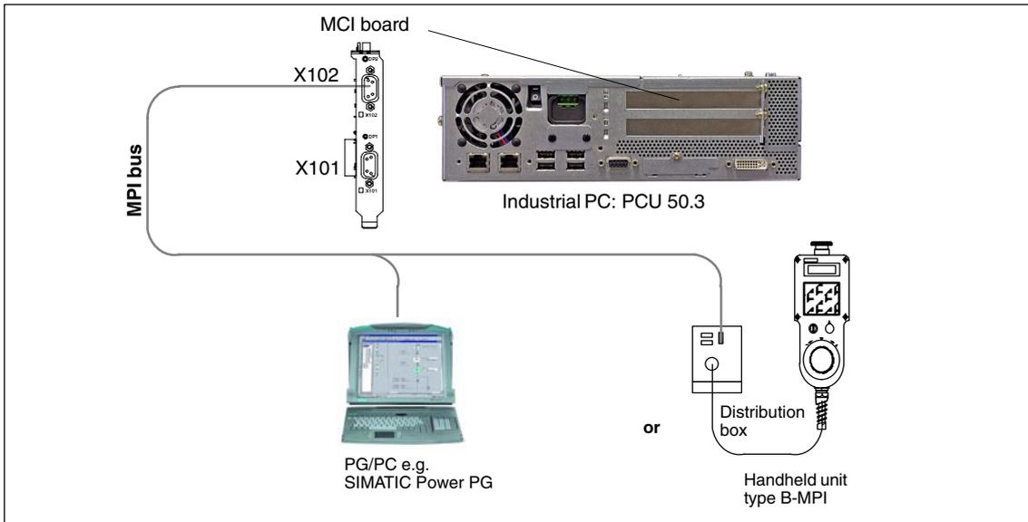
Fig. 3-3 System overview of SINUMERIK 840Di sl MPI (schematic)
