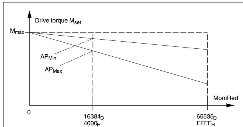
Fig. 18-6 Drive torque for the evaluation (drive parameter AP) and torque reduction (MomRed) (Not true to scale)
