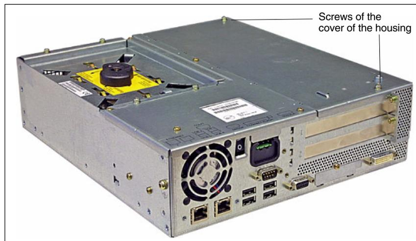
Fig. 2-8 Cover of the housing of the PCU 50.3
