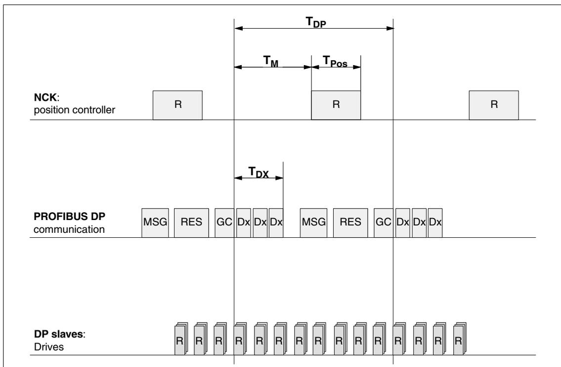
Fig. 11-2 Position control cycle offset compared to PROFIBUS DP cycle
