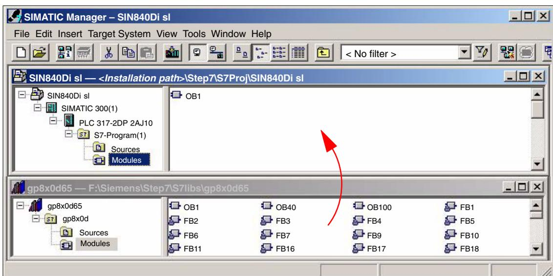
Fig. 6-7 Inserting blocks of the PLC basic program
