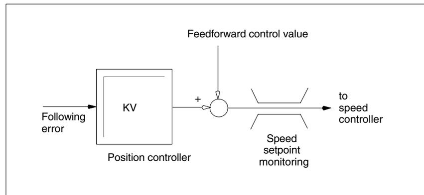
Fig. 11-21 Speed setpoint calculation
