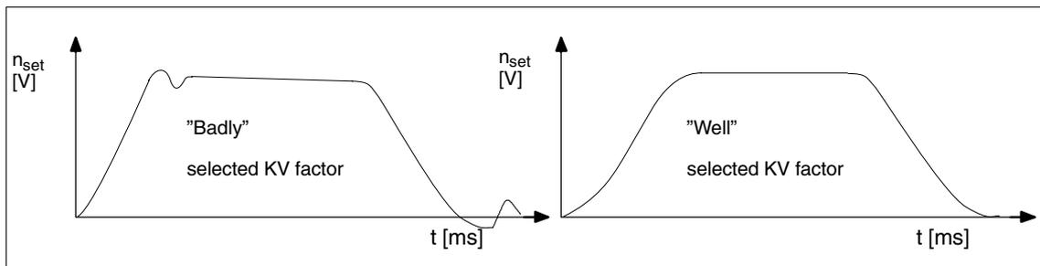
Fig. 11-17 Speed setpoint characteristic
