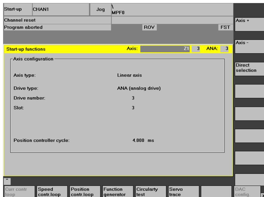
Fig. 3-3 “Start-up functions” menu display
